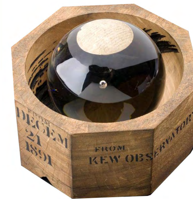
A Campbell sunshine recorder was a 19 th century meteorological instrument that utilized a glass sphere to focus the sun's rays and burn a record of clear or cloudy skies into a wooden bowl. Deployed from solstice to solstice, each bowl is an intriguing, informational and beautiful 6-month archive of solar conditions.
