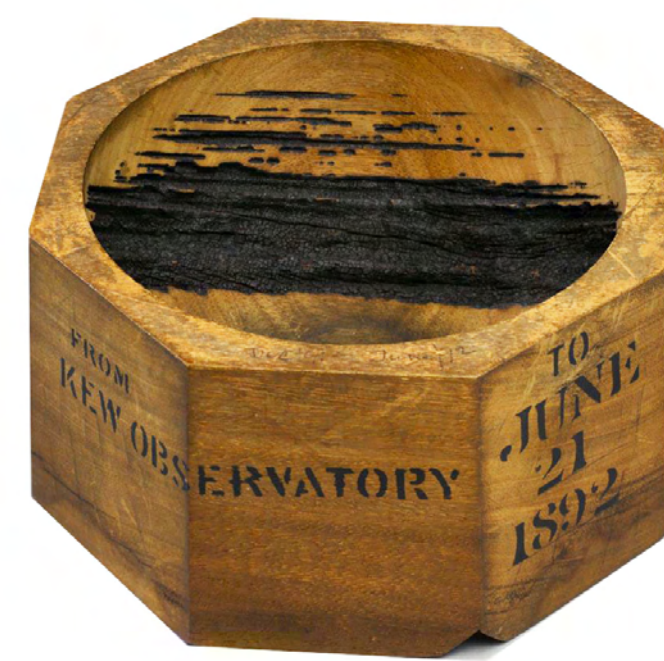
A Campbell sunshine recorder was a 19 th century meteorological instrument that utilized a glass sphere to focus the sun's rays and burn a record of clear or cloudy skies into a wooden bowl. Deployed from solstice to solstice, each bowl is an intriguing, informational and beautiful 6-month archive of solar conditions.
