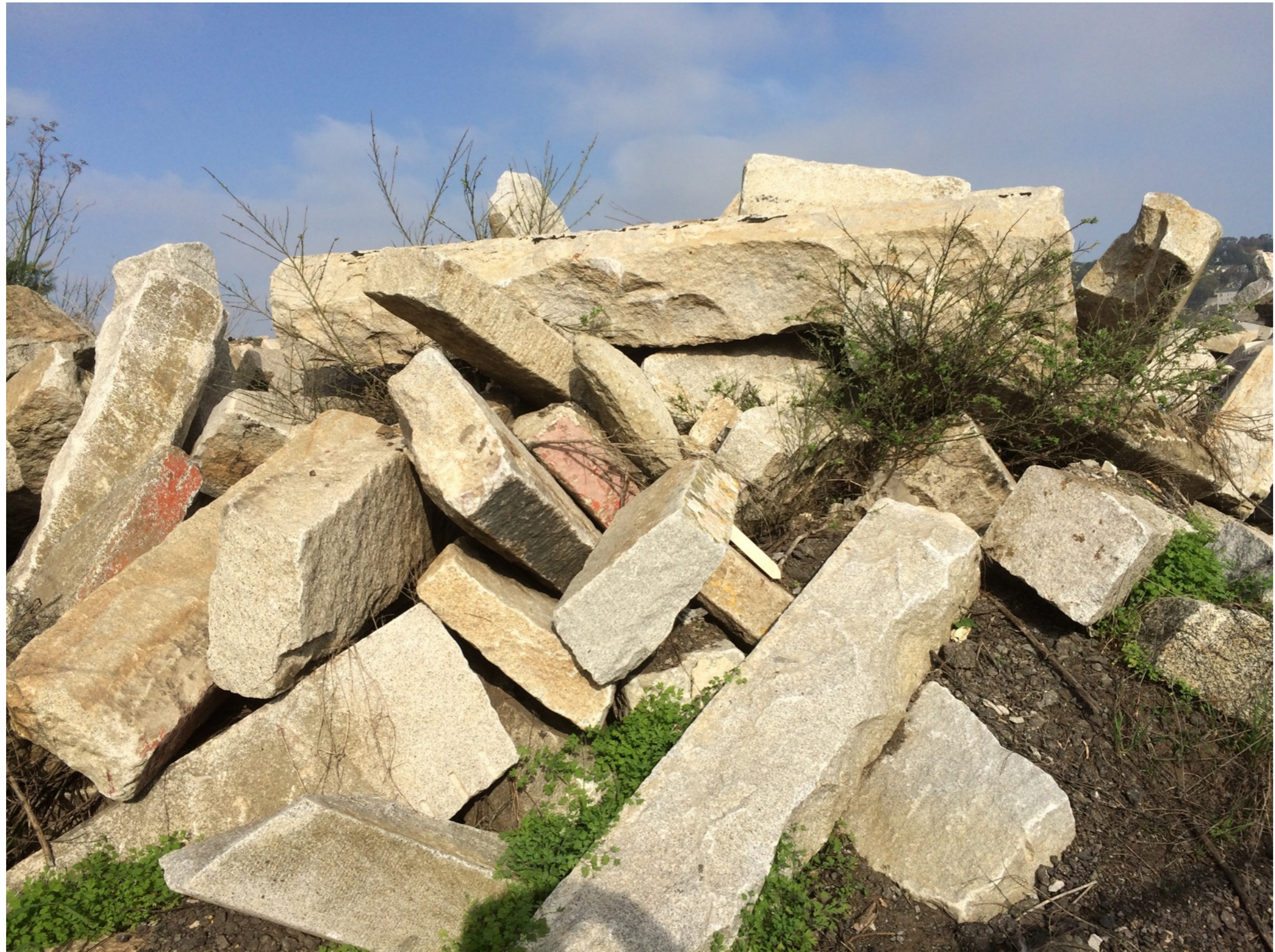
Reclaimed curbing from DPW
