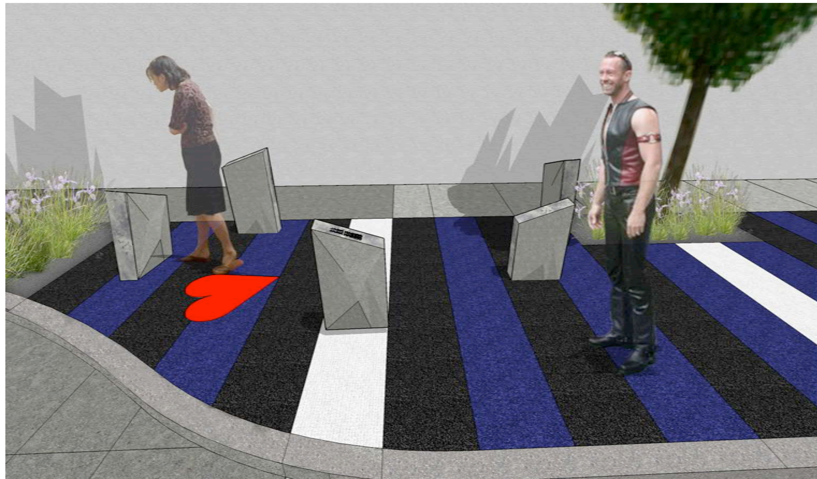
CONCEPT IMAGE: STANDING CURB STONES AT TRAFFIC CALMING CHICANE WITH PAINTED PAVEMENT
