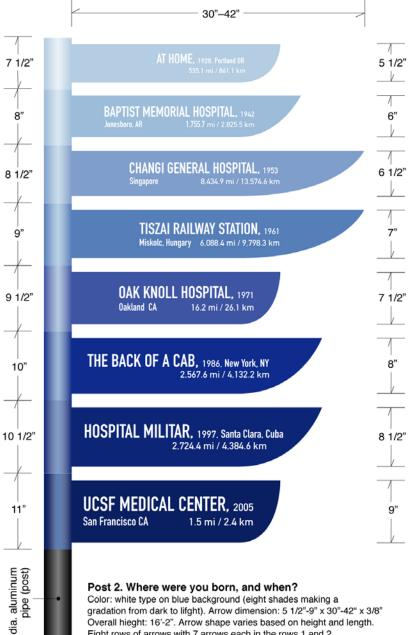
Overall hieght: 16'-2". Arrow shape varies based on height and length. Eight rows of arrows with 7 arrows each in the rows 1 and 2, 6 arrows each in rows 3 and 4, 5 arrows each in rows 5 and 6, and 4 arrows each in rows 7 and 8 for a total of 44 arrows/place names.
