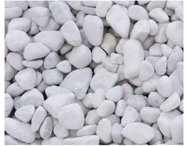
DECORATIVE LIGHT ROCK BALLAST (ROOF)
