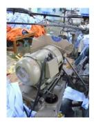
• Also in Building One, the drop cord of one sewing machine is pulled, conductors are exposed, and insulation is cracked.
