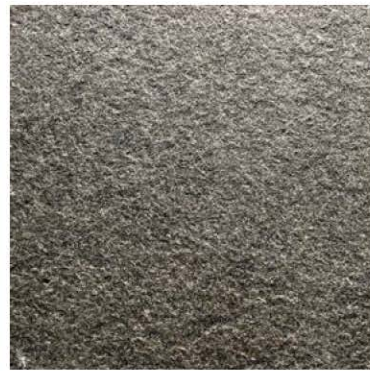
Cobble Alternate 3.5" x 3.5" x 1.5" Quarry House basalt Britannia Black Flamed Finish on top surface Sawn sides and bottom Mortar set on concrete subslab
