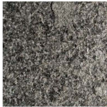
Granite Cobble 3.5"x3.5"x1.5" Coldspring granite Academy Black Thermal Finish on top surface Sawn sides and bottom Mortar set on concrete subslab
