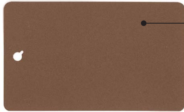
POWDER COAT ALUMINUM FASCIA/BEAM CLADDING (TEXTURED COR-TEN)
