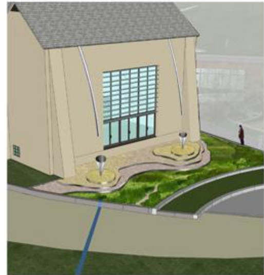
Detail showing downspout sculptures that filter and slow runoff. The topographical shapes are derived from the surrounding hills. The steel shapes are filled with native gravel (Chert) and can be planted with groundcover.
