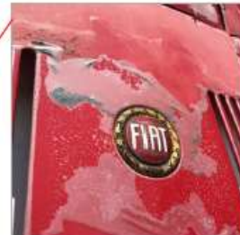
Figure 3: Deteriorated clearcoat with atmospheric soiling trapped inside. Faded red powder coating.
