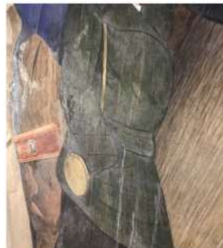
Figure 21: Detail of glossy film and white drips on a different area of the Powell Street mural.
