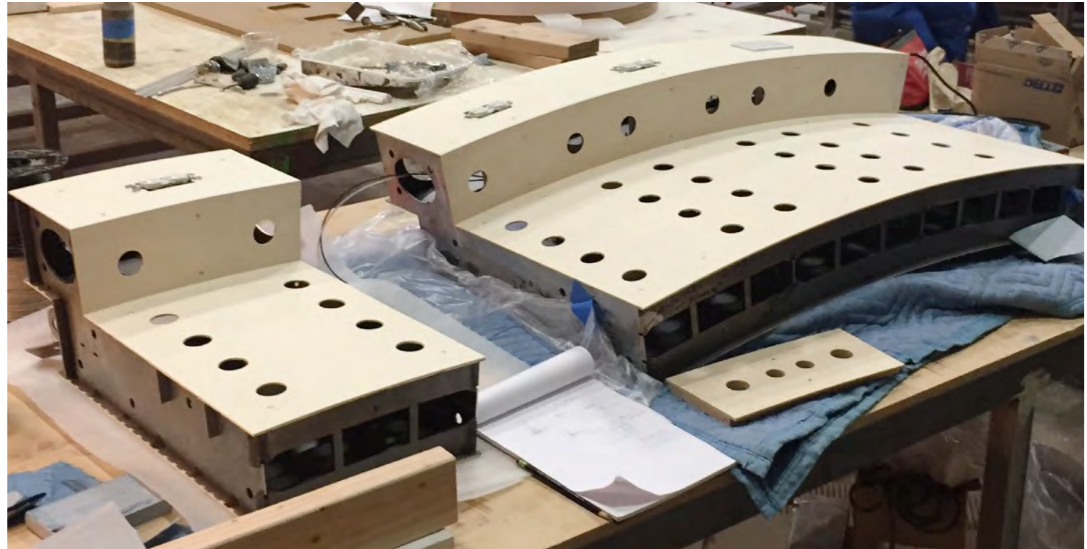
Construction technique for top structure: metal skinned with bendy poplar
