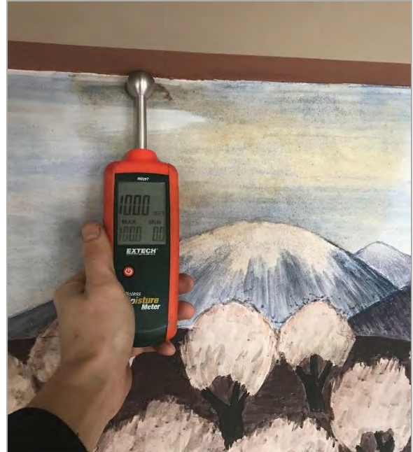
Figure 4: Detail of a reading taken at above the door frame at the California mural. Image shows 100% water content on the wall.
