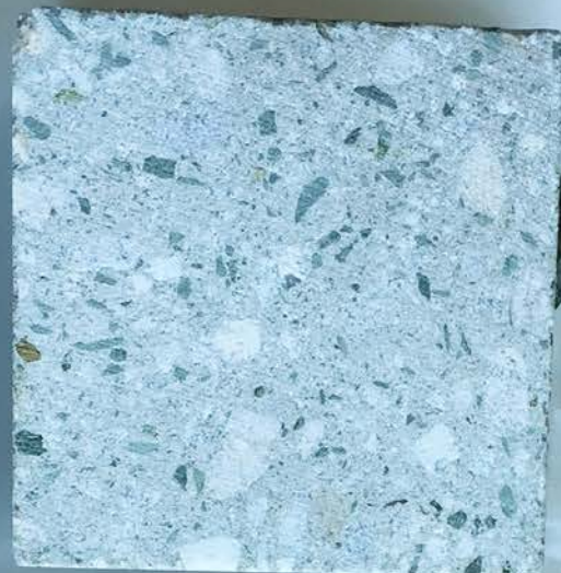
Ground concrete finish for plaza.
