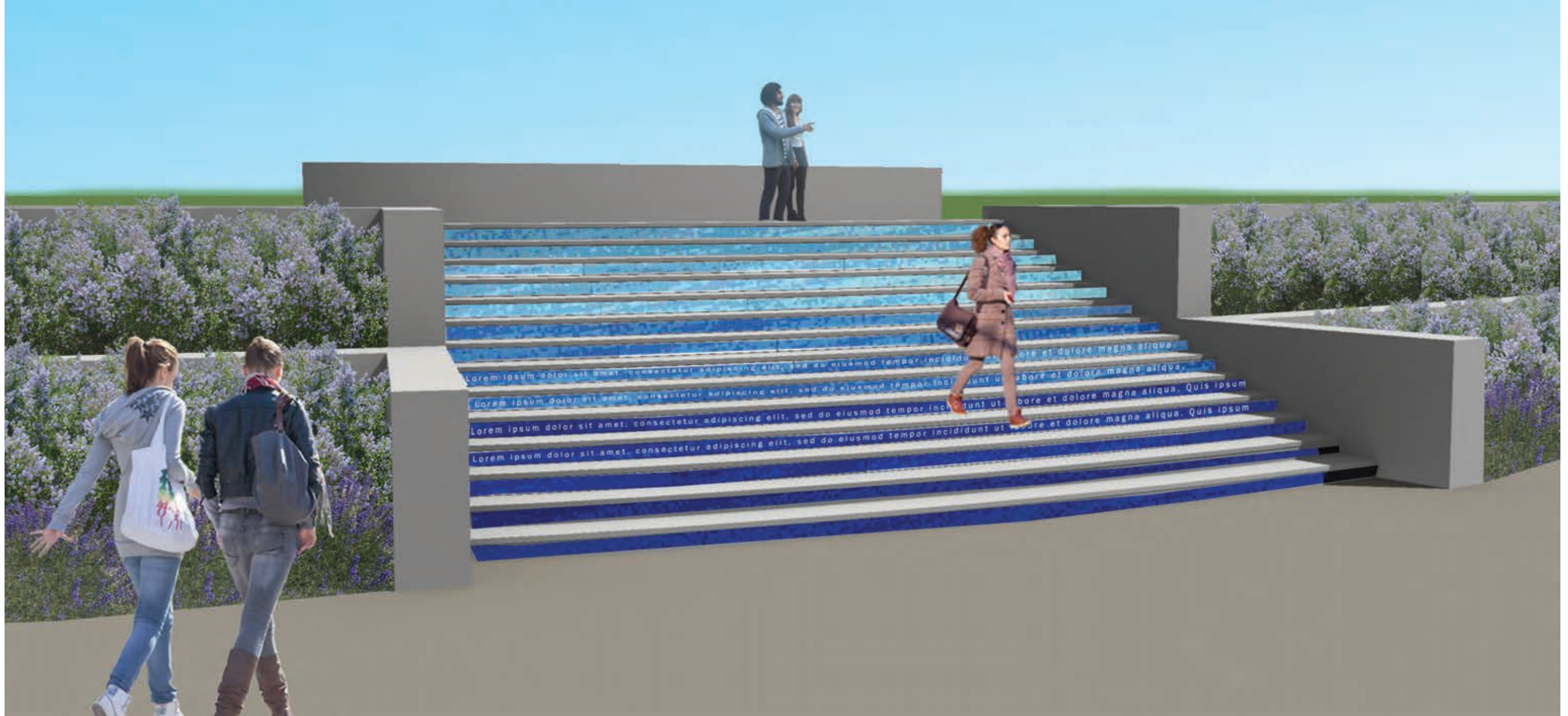
Donor Steps - Colored metal plates recessed into step risers with etched donor names. Plates fastening with tamper proof screws so they can be removed to add additional names in the future. Final plate size and color TBD.
