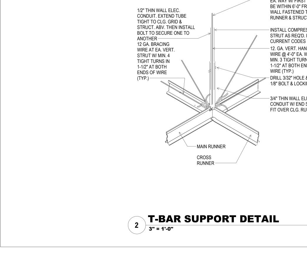
**CLG. INSTALLATION MUST BE IN ACCORDANCE W/ THE PROVISIONS OF ASTM C635** & C636
