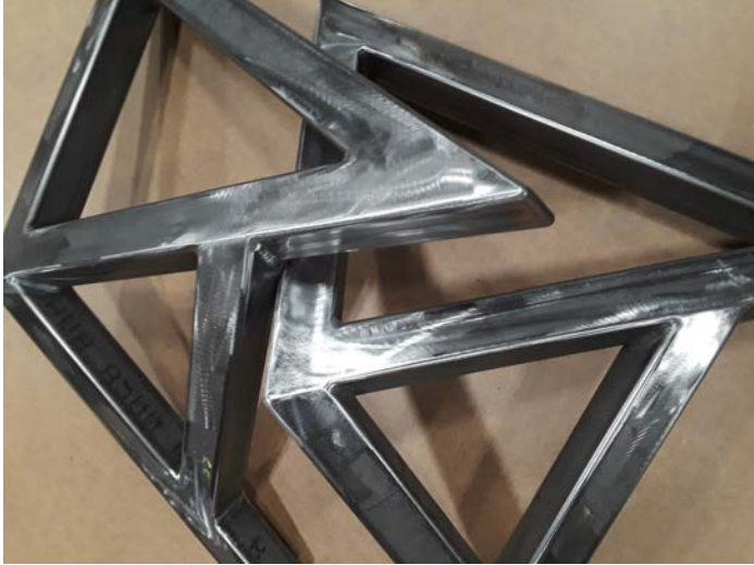
Fig. 11 Welded steel sample parts prior to finishing
