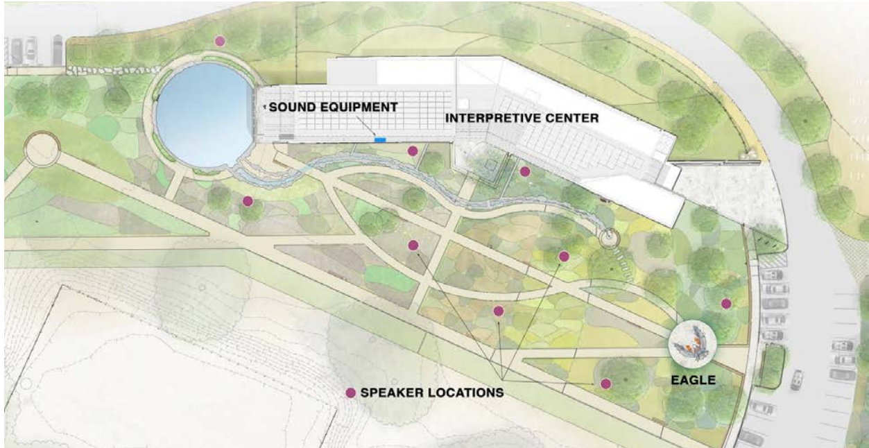
Fig. 15 Speaker Locations - audio cables are below ground in conduit. Control panel in building.
