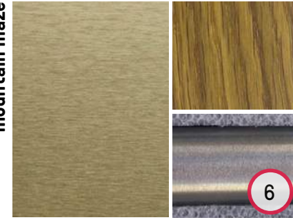
6 Mesh: GKD Futura 3110 -SSL Road: Natural Anodizing Aluminium Structure: Gunmetal Grey Steel
