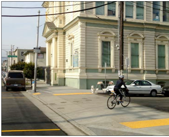
RAISED CROSSWALK WITH FEATURE PAVING
