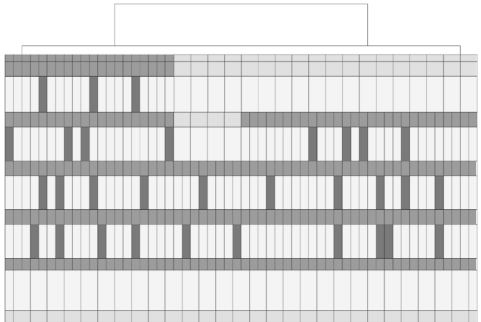
NORTH ELEVATION: 31 SOLID PANELS
