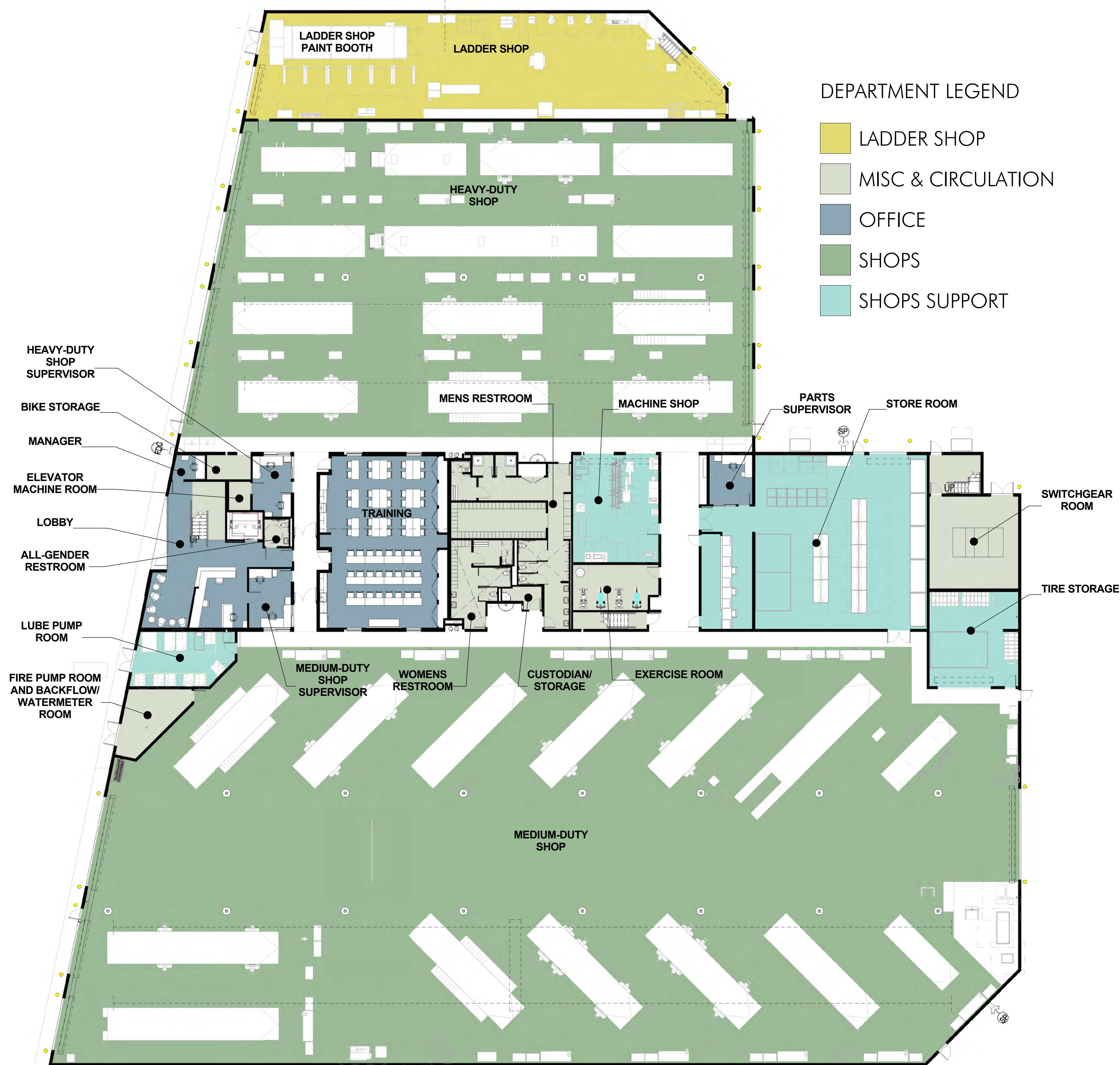
1 FIRST FLOOR PLAN 1/16" = 1'-0"
