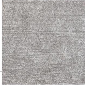
Concrete Curb 2 lbs/CY Lamp Black Added
