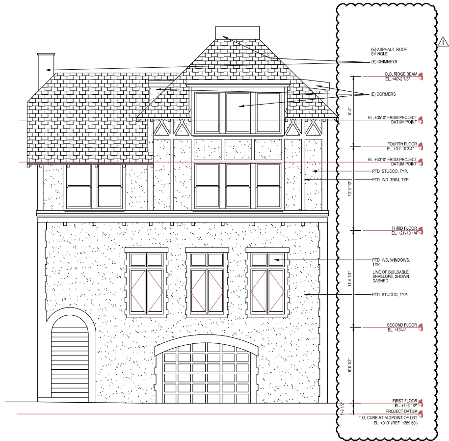
EXISTING EAST ELEVATION
