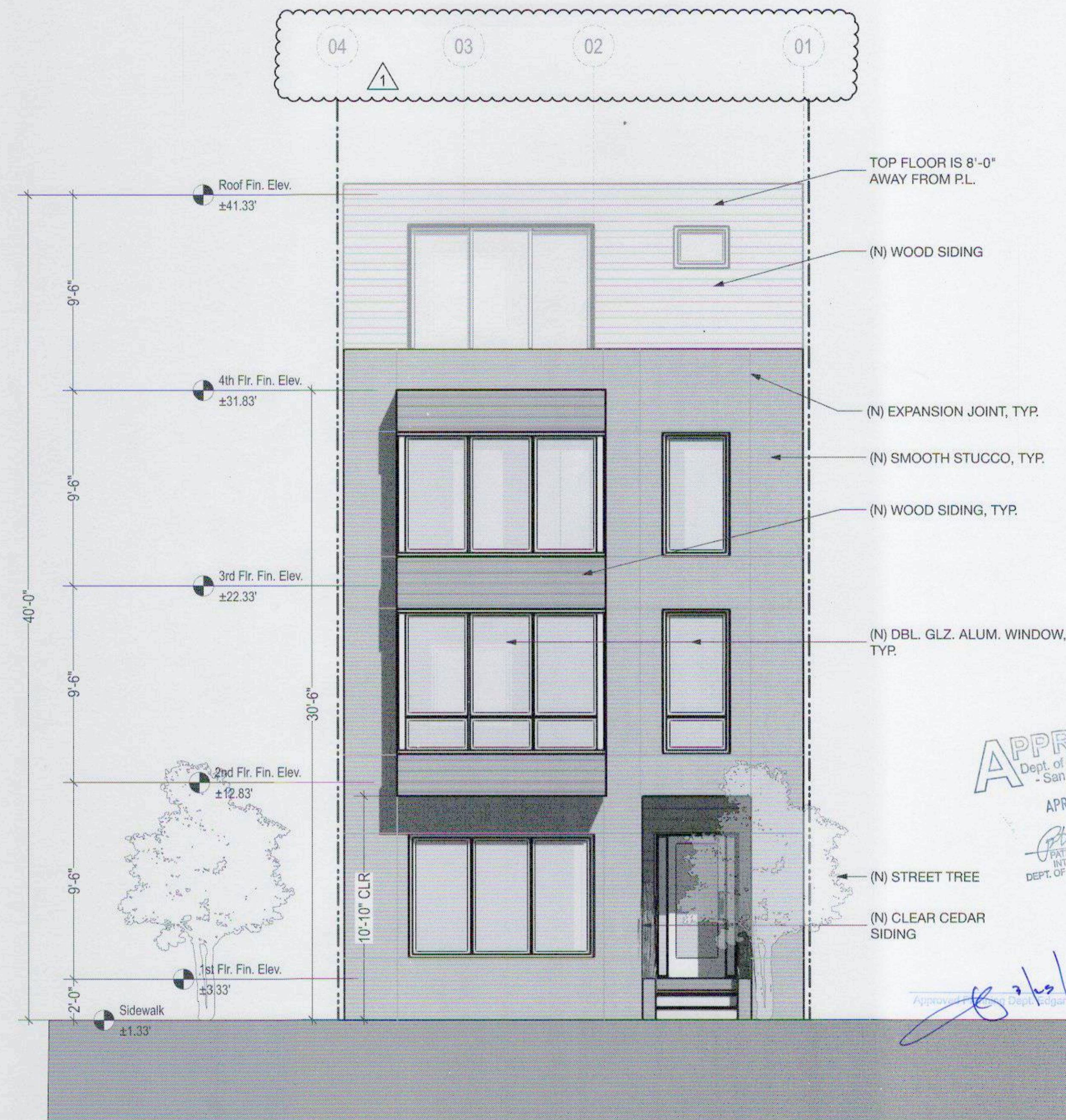
Proposed Front Elevation, Rear Addition (South) 1/4" = 1'-0"
