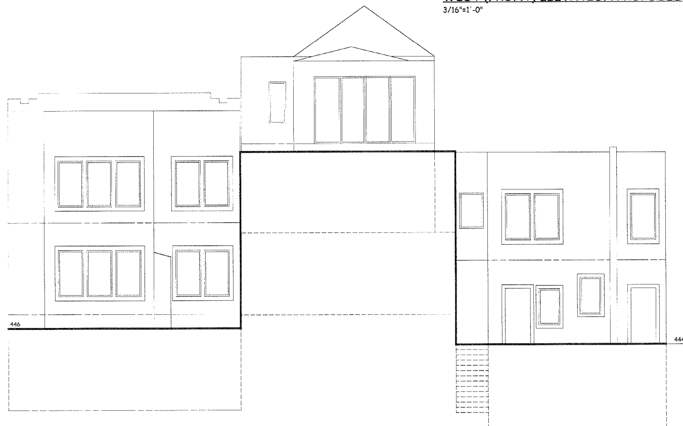
WEST (FRONT) ELEVATION PROPOSED 3/16"=1'-0"
