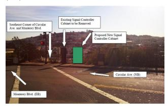
Controller cabinet is 36"W x 60"H x 17"D; Concrete foundation is 38"W x 6"H x 19"D Total Height (cabinet & foundation): 66"
