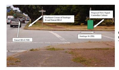
Controller cabinet is 36"W x 60"H x 17"D; Concrete foundation is 38"W x 6"H x 19"D Total Height (cabinet & foundation): 66"
