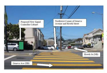
Controller cabinet is 36"W x 60"H x 17"D; Concrete foundation is 38"W x 6"H x 19"D Total Height (cabinet & foundation): 66"
