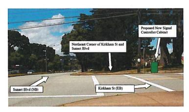
Controller cabinet is 36"W x 60"H x 17"D; Concrete foundation is 38"W x 6"H x 19"D Total Height (cabinet & foundation): 66"
