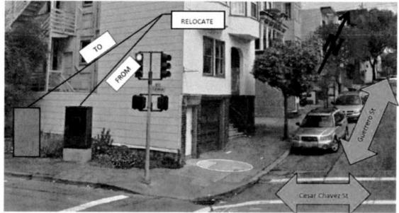
Controller cabinet is 36"W x 60"H x 17"D Concrete foundation is 38"W x 6"H x 19"D Total Height (cabinet & foundation): 66"
