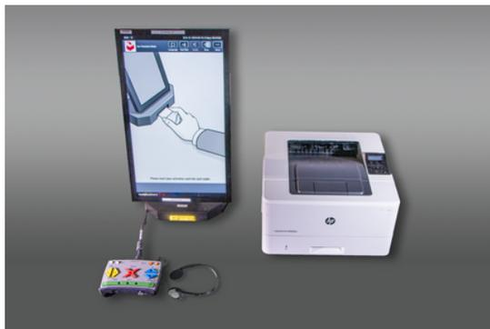
device have the option to view or hear a summary of their choices and change any selections before printing their ballots. The ballot-marking device only marks a ballot; it does not count votes. The device generates and prints a paper ballot with the voter's selections. The ballot is then scanned through the Ballot Scanner at the polling place for tabulation.
