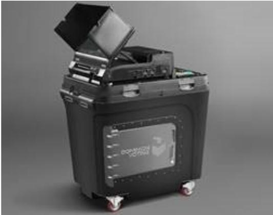
Every polling place will have provided with an ImageCast Evolution Ballot Scanner, an optical scan tabulation machine that scans and tallies voted ballots. The equipment scans a full digital image of the marked ballots and counts the votes electronically. The ballots are then deposited into a sealed ballot box.
