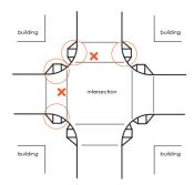
When performing any excavation in any portion of the crosswalk, evaluation of the angular returns of the affected crosswalk is required. If curb ramps do not exist or are not constructed per current DPW Standards, curb ramps shall be constructed by excavator to complete the path of travel at all returns in the intersection.
