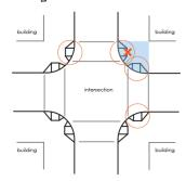
When performing any excavation within the public right of way, affecting any portion of the angular return, evaluation of the cross-walk(s) adjacent to the affected angular return is required. If curb ramps do not exist or are not constructed per current DPW Standards, curb ramps shall be constructed by excavator to complete the path of travel from that angular return.
