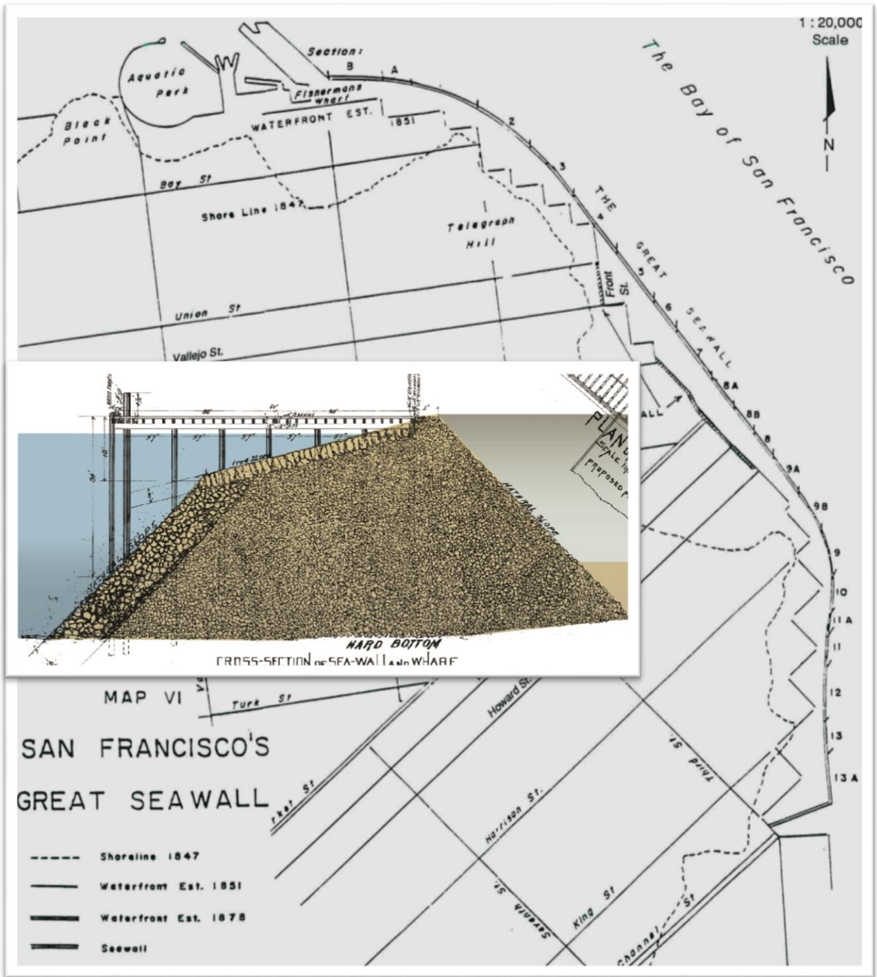
FIGURE 6. MAP OF THE SEAWALL SECTIONS ALONG SAN FRANCISCO'S EASTERN WATERFRONT AND A COLOR-ENHANCED CROSS-SECTION OF SECTION 12 OF THE SEAWALL CIRCA 1907
