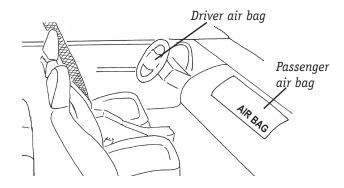
All cars since model year 1998 must have both driver and passenger air bags. Both air bags are required in all pickups, SUVs, and vans starting in the 1999 model year. Many vehicles made earlier in the 1990s have air bags, too. Check the owner's manual and look for the letters on the dashboard and the warning on the sun visor.
