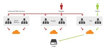
An attacker gathers resources, such as botnets or unsecured DNS recursors, and imitates the target's IP address. The resources then send a flood of replies to the target, but they are blocked by Acquia Cloud Edge Protect's data centers. Legitimate traffic can still access the web property.
