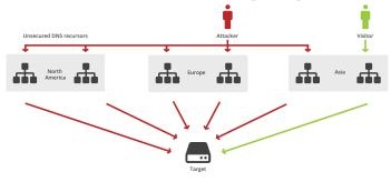
An attacker gathers resources, such as botnets or unsecured DNS recursors, and imitates the target's IP address. The resources then send a flood of replies to the target, knocking it offline.
