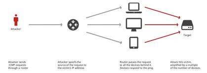
SMURF attacks are largely a thing of the past. For the most part, network operators have configured their routers to disable the relay of ICMP requests sent to a network's broadcast address.
