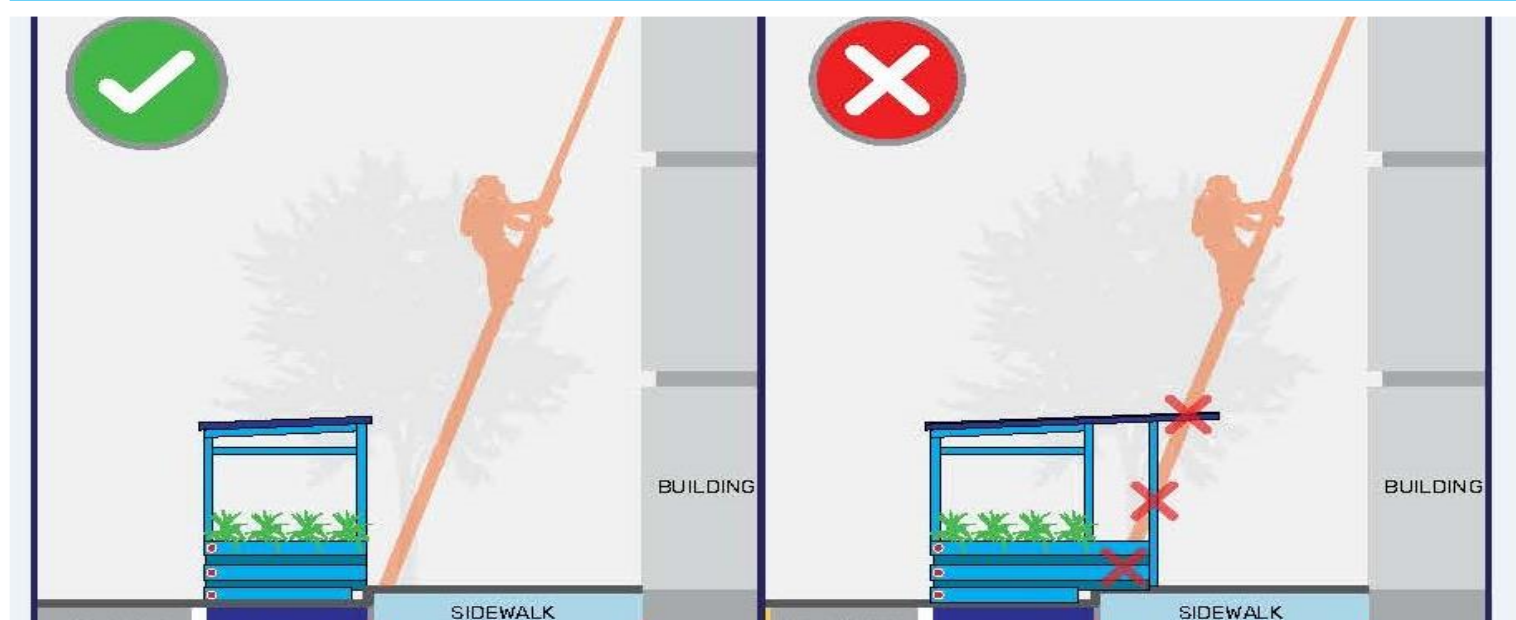
Clearance for Firefighting Ladders
