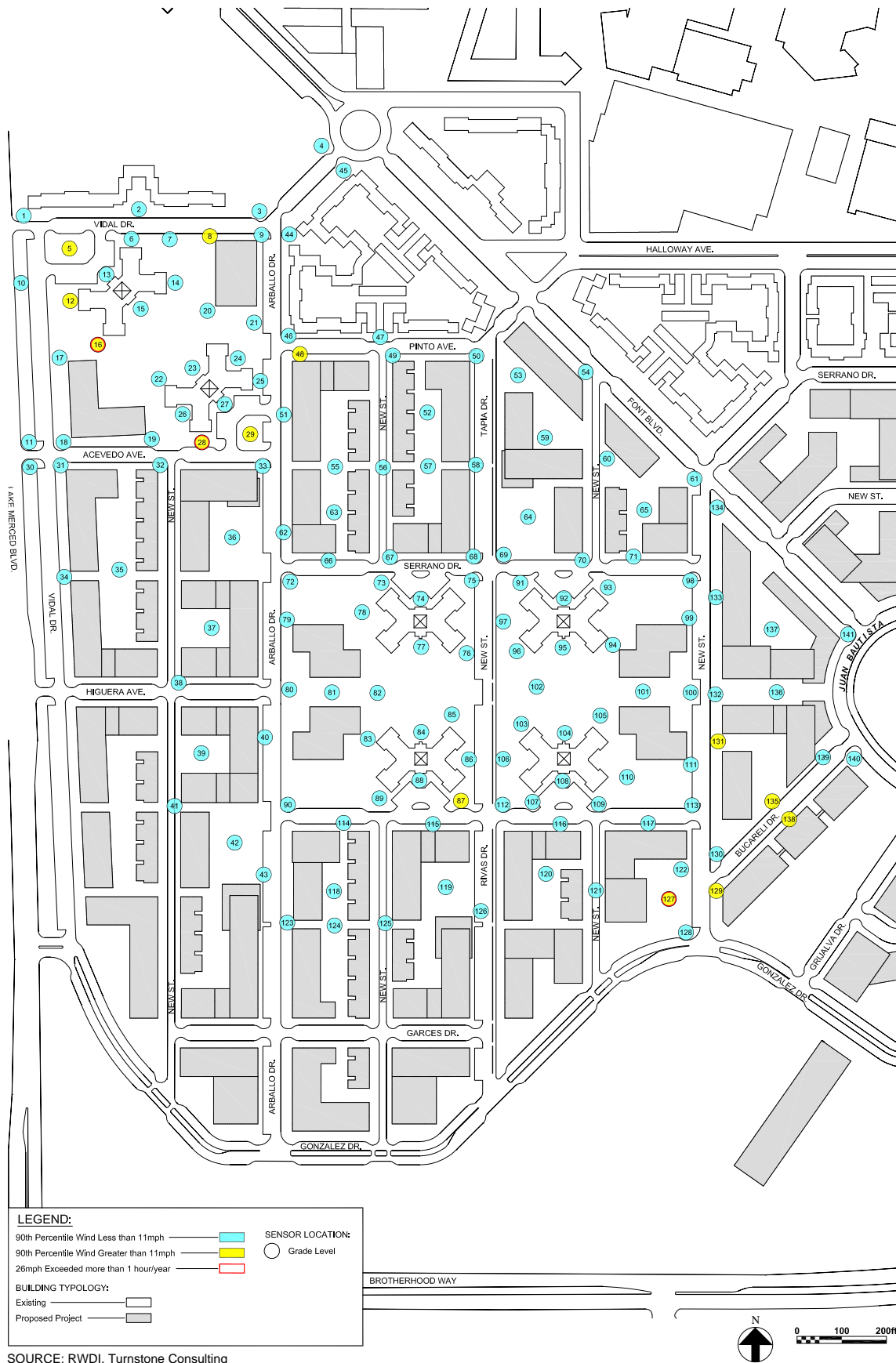
FIGURE V.I.3: WIND TUNNEL TEST POINT LOCATIONS – WEST SIDE PROPOSED REPRESENTATIVE PROJECT CONFIGURATION
