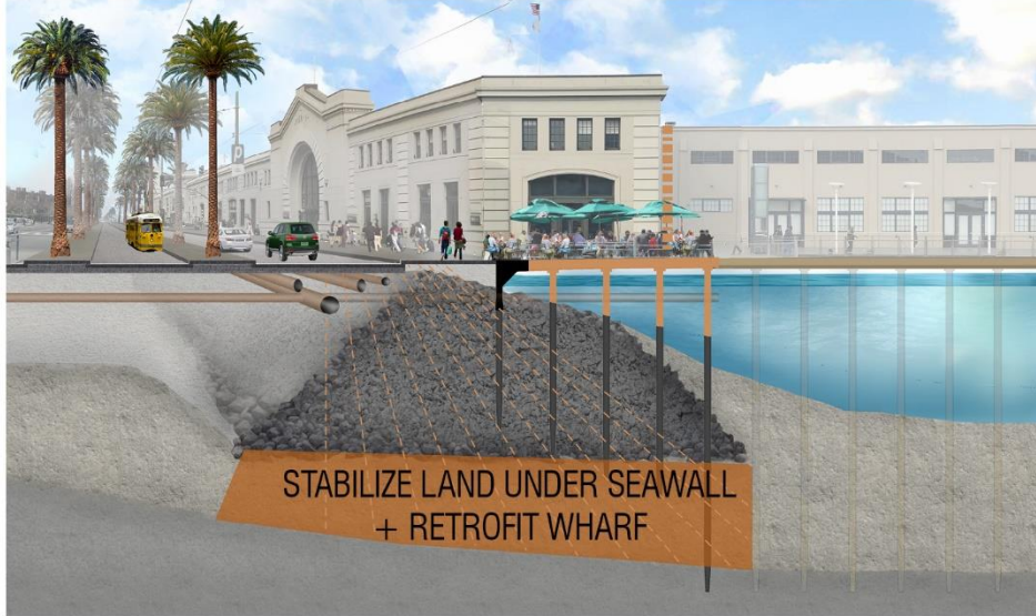
OPTION 2 GROUND IMPROVEMENT UNDER SEAWALL
