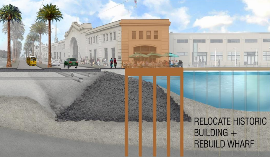
OPTION 3 BULKHEAD REPLACEMENT
